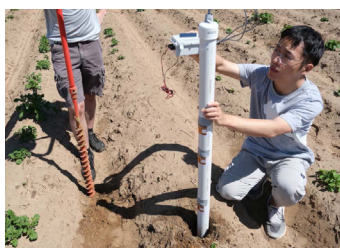
Shuohao Cai places a sensing rod with multifunctional sensing stickers enabling multi-depth measurements to test the team's tech. at Hancock ARS. Photo by Kuan-Yu Chen
